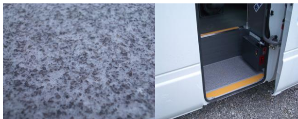
Fig.1 The Image of Non-Slippery Floor Material 表1 新しい床材のすべり抵抗値(CSR値)測定結果 Table.1 The Evaluation of CSR of New Material
